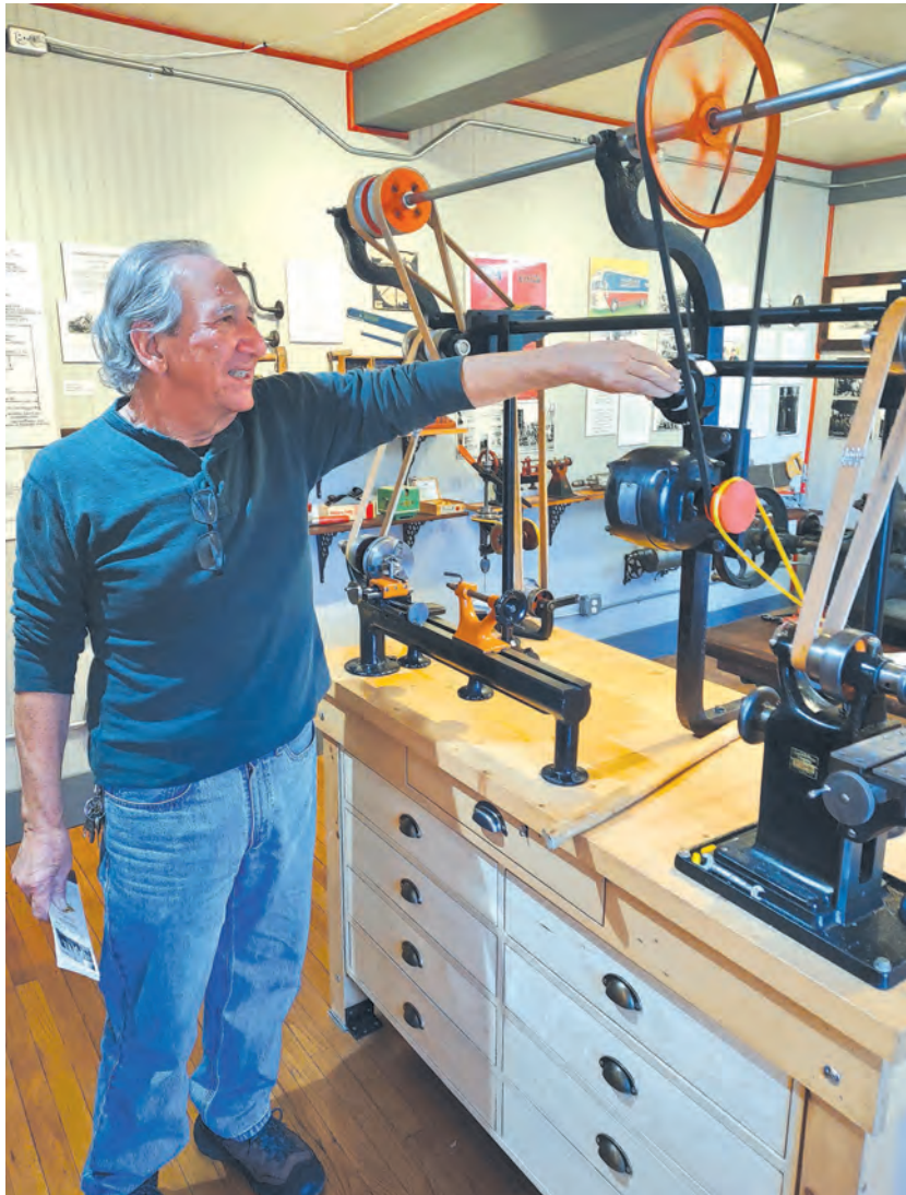
Jim Terapane operates the Goodell-Pratt Company’s “light shop equipment with motor drive,” the only example of its kind remaining in the world.
