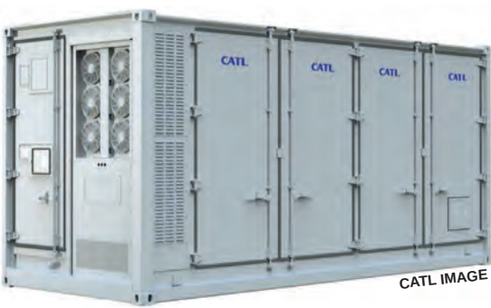
The applicant hopes to install a single CATL EnerX unit – the 20-by-8-by-10-foot container pictured above – at its proposed solar array. The unit includes its own thermal management and fire suppression systems, but if these fail there is some risk of a “runaway” fire that cannot be extinguished with water.
