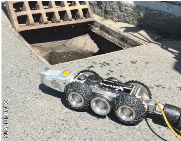
The town’s remote-controlled robotic camera can burrow through subterranean pipes, providing staff with a live feed showing their condition and allowing the department to identify sites of groundwater infiltration, a perennial challenge aging collection systems pose to wastewater management.
