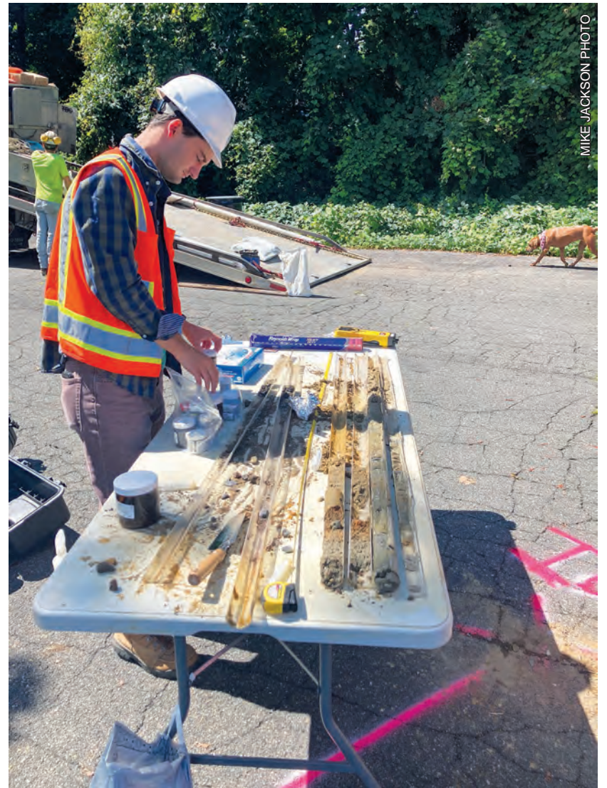
A US Department of Transportation employee, contracting with the Environmental Protection Agency, gathered samples on August 1 for a Phase II environmental assessment of the First Street lot slated for new Habitat for Humanity housing. A separate drilling crew helped make six borings for soil samples, as well as two monitoring wells. As it turned out, the soil contained low levels of six toxic chemicals.
