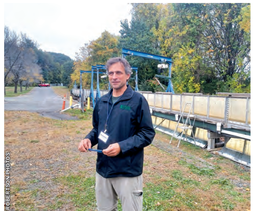
Conte Lab research ecologist Ted Castro-Santos stands in front of a demonstration experiment at Saturday's open house: a flume in which he is measuring how effectively various species of fish swim against water flowing at different rates. "We just gave them four hours to see what they could do against about a meter-per-second flow velocity," Castro-Santos reported. "The answer was absolutely nothing."
