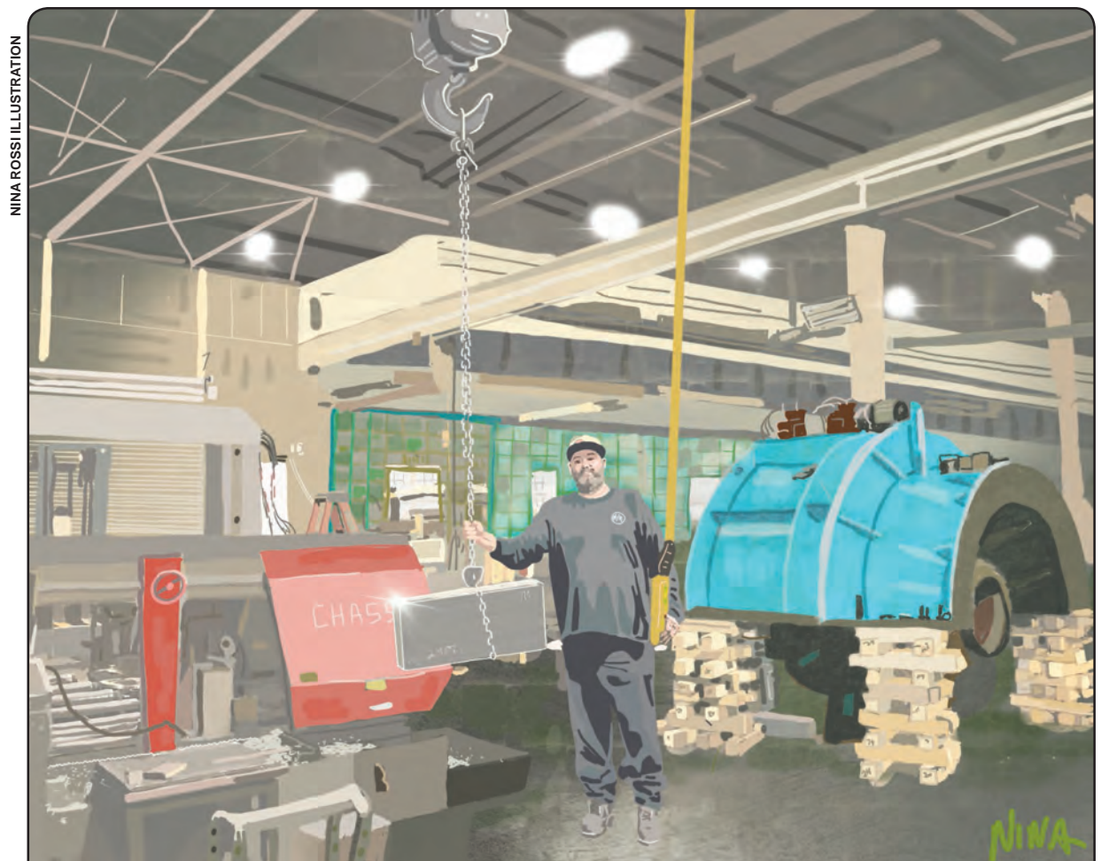
Adam Stockwell lifts a 271-pound block of titanium with one of the movable chainfalls inside Montague Machine on Rastallis Street in Turners Falls. The block is going to Wyman-Gordon, a firm that makes parts for the aerospace, energy, and military naval markets. At Adam's left is a hydroelectric turbine the company is rebuilding for a plant in Hillsborough, New Hampshire.
