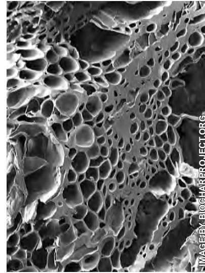
An electron microscopy image of biochar's sponge-like structure.
