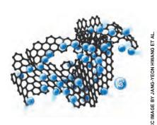
A depiction of sodium ions intercalating into a "hard-carbon" anode.
