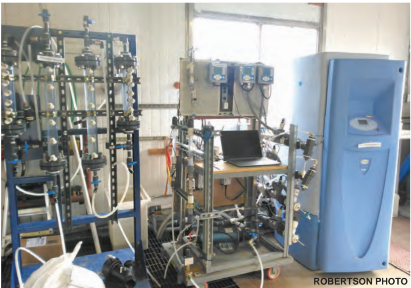
Equipment at the WET Center's main building, including a reverse osmosis machine (at right), is used to analyze PFAS and determine how to remove them from water.
