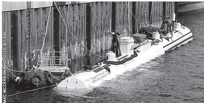
A tidal turbine moored at Hatston Pier in the Orkneys, Scotland.
