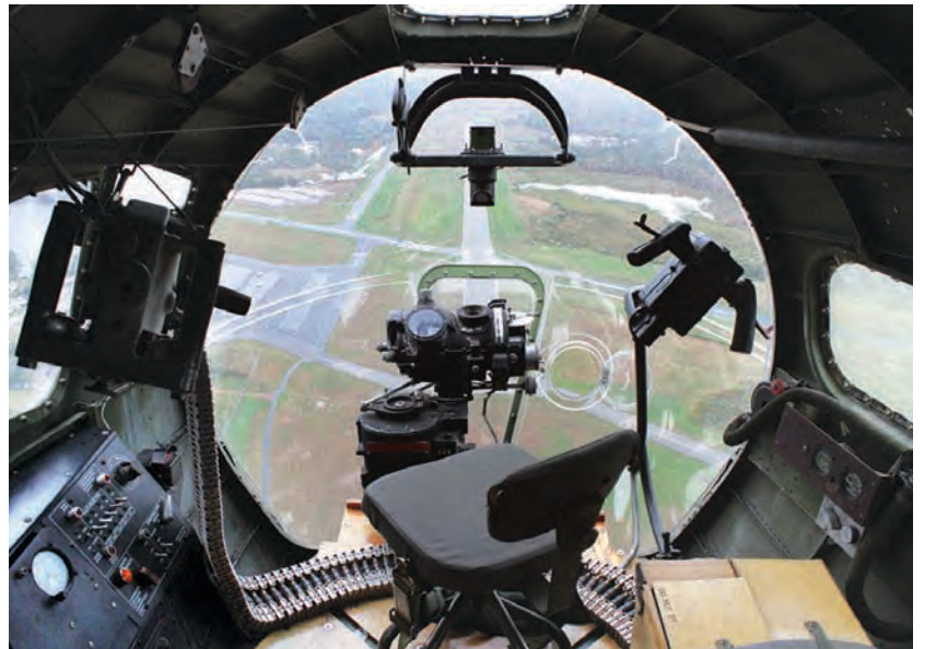
The Flying Fortress's chin turret, complete with a nine-yard clip of ammunition.
