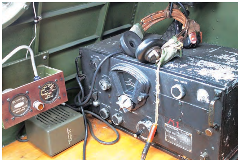
The radio operator's tools of the trade, including headphones and the oxygen gauge.
