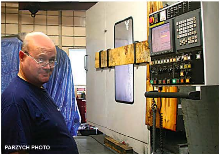
Tom Tyler operates a computerized SMK horizontal boring machine, boring holes into cast iron plate at the Montague Machine Co.
