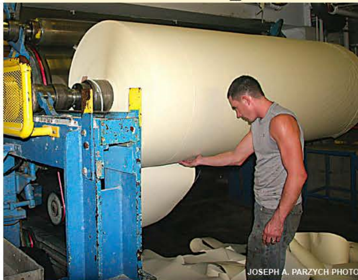
Ed Prondecki prepares a roll of paper for wrapping to ship to Southworth's finishing plant in Agawam
