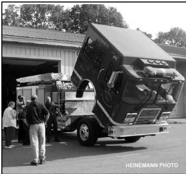
No, it's not broken. Wendell's new 2006 Smeal pumper features a tilt front end that allows for easier access to the 390 hp Cummins Diesel powerplant that drives the machine.
