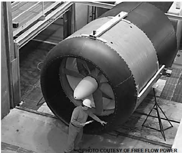
Ed Mamo, of EVP Power, inspects Free Flow Power's hydrokinetic turbine at the Conte Lab
