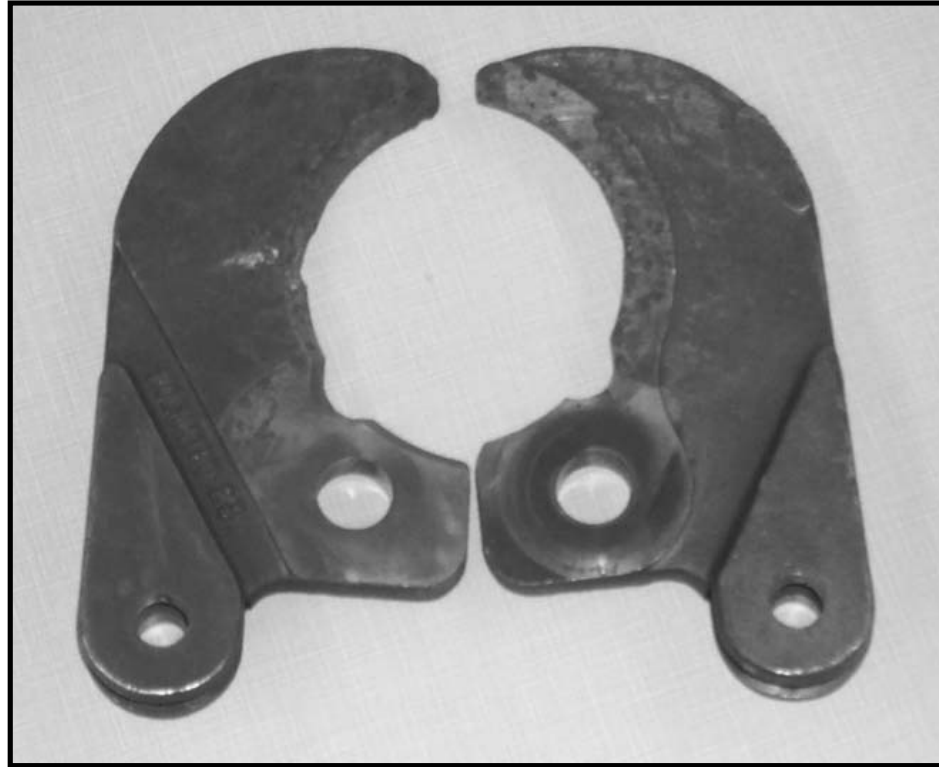
The cutting blades from the Jaws of Life failed to pass inspection due to a crack in the steel. Fire Chief Gene Beaubien estimates replacement costs at $3,250.
