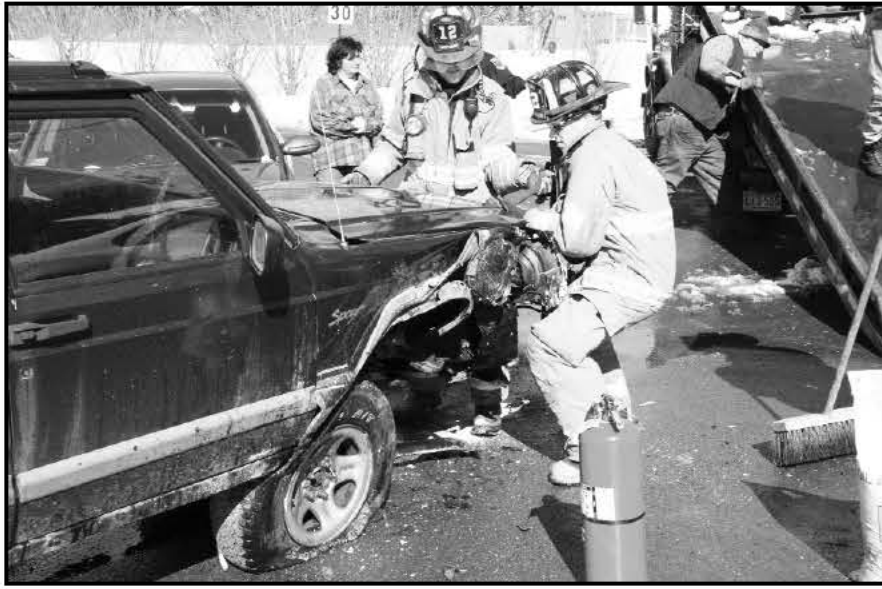
Photos and story by roving reporter Joe Parzych, author of Jep's Place . Pictured: Gill firefighters attempt to open Jeep Sport hood to disconnect the battery to avoid a short circuit starting a fire.
