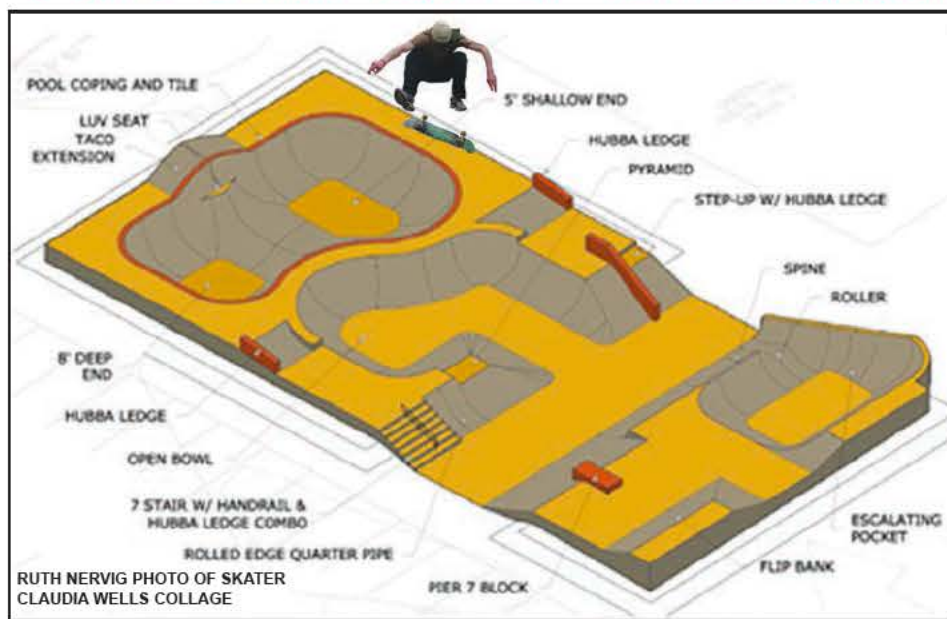
Schematic for the proposed skate park at Unity Park - from Pillar Design, Tempe, AZ
