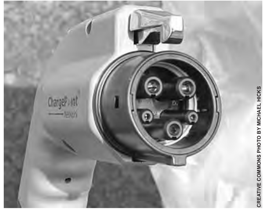
Most electric vehicles have this standard SAE J1772 charging connector.
