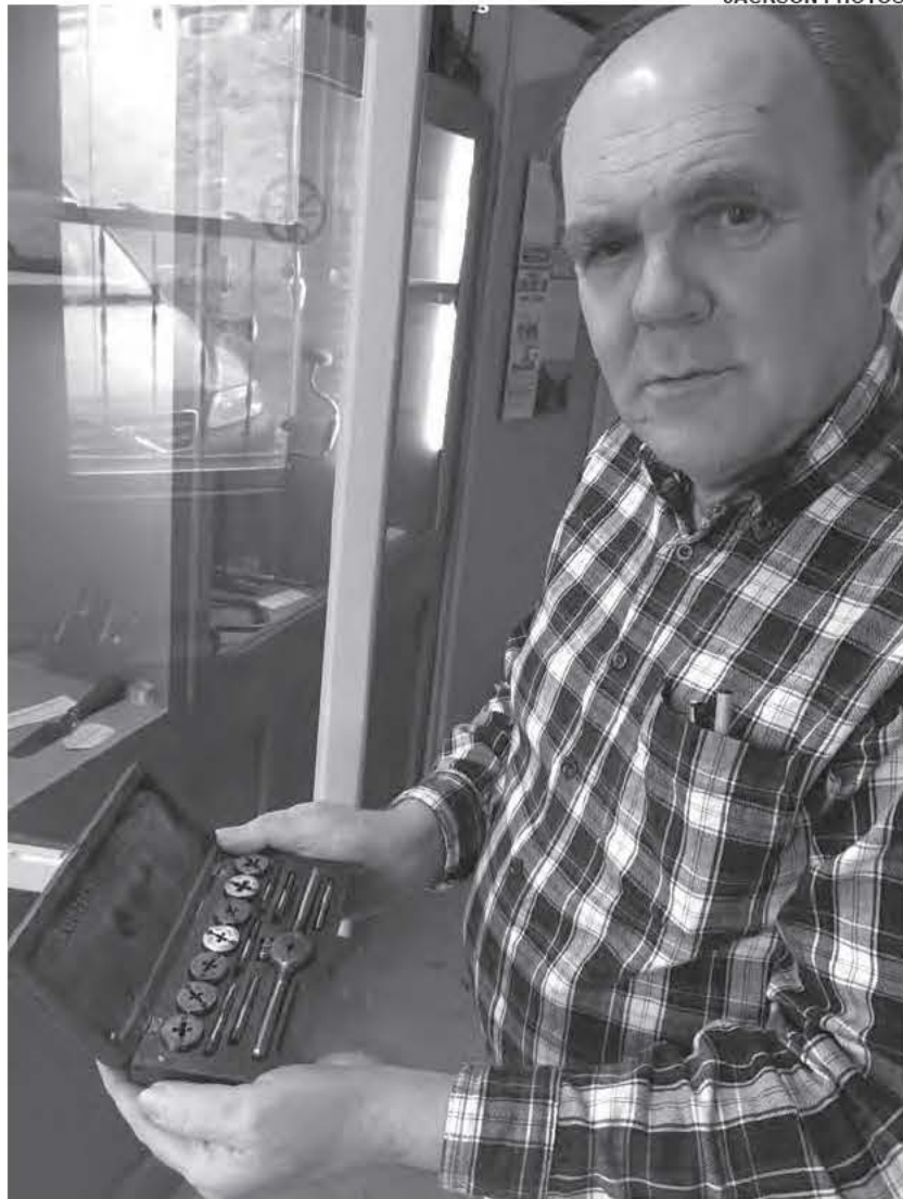
Chris Clawson shows off one of the Museum’s early tap and die sets, manufactured nearby by the Wiley & Russell Manufacturing Co. under an 1877 patent.
