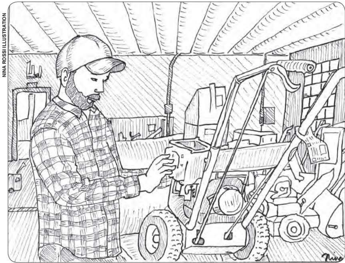
Mechanic Mike Douglass works on one of 30 snowblowers awaiting seasonal maintenance at Sirum Equipment in Montague. Mostly, he says, the carburetors are gummed up by ethanol from pump gas. Running a quart of ethanol-free gas before storing any engine is highly recommended. (It goes for $8 a quart at Sirum's!)
