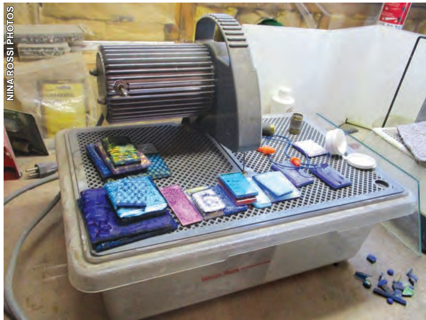
Smaller pieces of glass arranged on the ring saw that Ina uses for cutting more intricate shapes.
