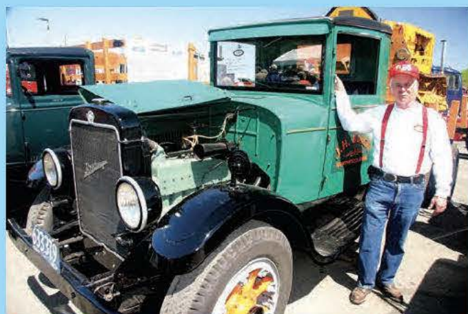
John H. Black of Northfield showed his 1929 Reo Speedster with only 49,000 actual miles on the speedometer. The engine appears to be a Continental, sporting seven main bearings. The truck was purchased new by Gordon Gerry of Warwick, and has been operated as a log truck ever since, though occasionally carrying a Caterpillar logging tractor like the one aboard. Black did all the restoration but the lettering on the door.
