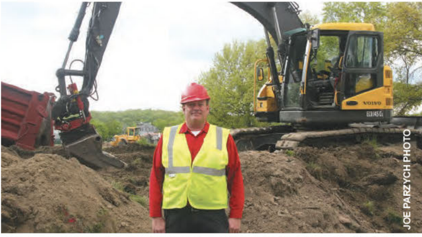
Taylor Davis stands in front of his Volvo ECR 145 CI Excavator. The bucket can tilt and revolve 180 degrees.
