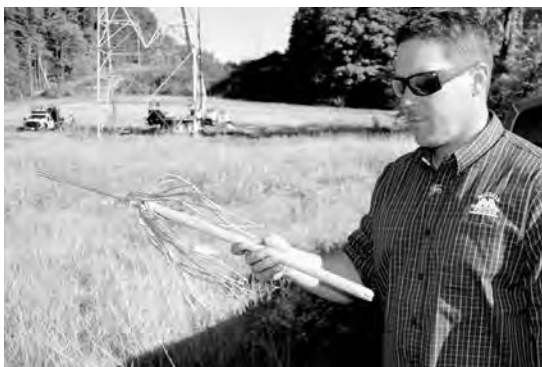
Michels Power Hi-line General Foreman Zack Landmark holds a section of aluminum high tension line equipped with composite ceramic core. The outer aluminum wires are flexible, but the composite core lines are as brittle as uncooked spaghetti.
