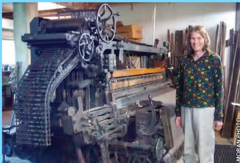
Peggy Hart with one of her looms. The abacus-like structure at the end of the loom is called the "pattern chain." It can be manipulated to make changes within patterns, or replaced with another one for a significant design alteration.
