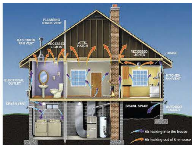
Illustration of the Stack Effect EPA image.
