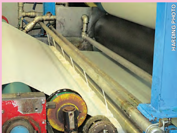
Finish treatment is added to the paper at the newly renamed Turners Falls Paper mill.
