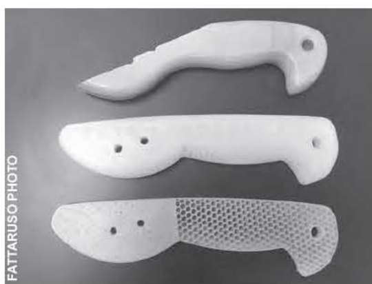
This broken saw handle (top) can be replaced with parts made on the 3D printer (below).
